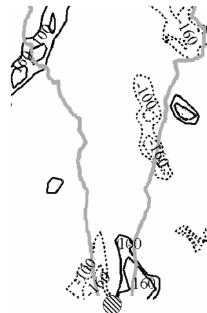
Fig. 4 Instantaneous vorticity contours (solid line, positive vorticity; dashed line, negative vorticity) along with flame front edge (gray solid line) of a stable flame at \phi = 0.72 (flow direction is from bottom to top).
